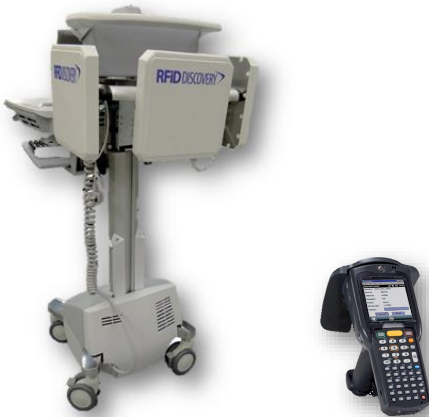
Figure 3: Mobile RFID reader and hand scanner.
