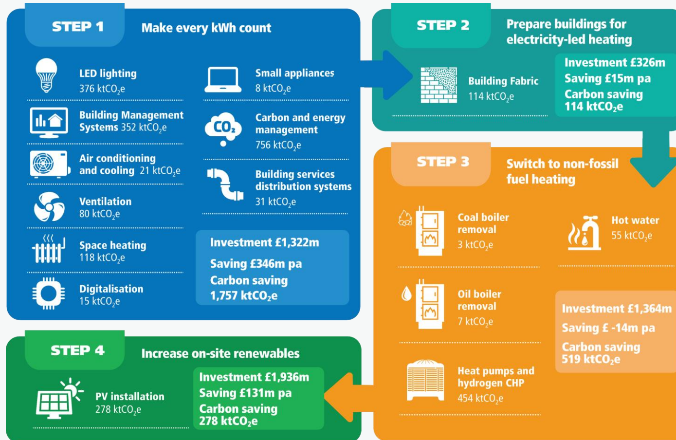
Figure 1 includes indicative numbers to illustrate the scale of the challenge to decarbonise the NHS estate by 2040. These are not actuals.
